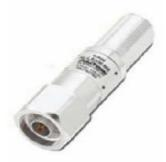
Filter technology is the simplest and most effective type of RF protection. The AWSAL-LSXM-ME PolyPhaser Lightning Protector appears as a short-to-shield on the surge side and is open between ports. It is optimized to pass the desired perating frequencies while attenuating lightning and dc components.
